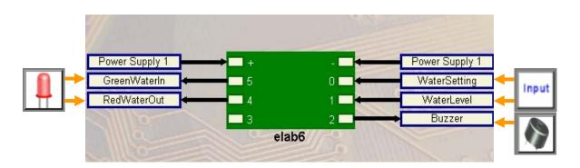
Use ezCircuit Designer to construct an input/output (I/O) diagram
