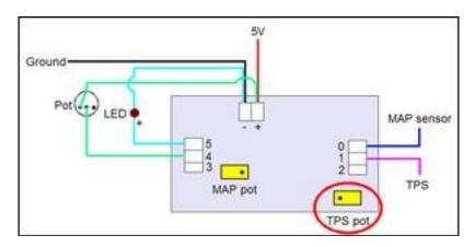
In this diagram the TPS setting pot is highlighted.
