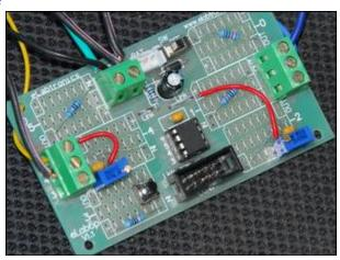
FuelS mart is based on an electronic module produced by Australian electronics company, eLabtronics. It uses a custom programmed microprocessor, a dash-mounted LED, two set-up pots, one remote-mounted fine tuning pot, and a pushbutton. It costs AUD\$45 (+ GST for Australian buyers = \$49.50) and can be bought directly from eLabtronics – see the link at the end of this article.
