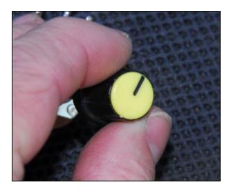
The external pot allows easy fine-tuning of the main MAP pot setting. The external pot is provided for three reasons:
