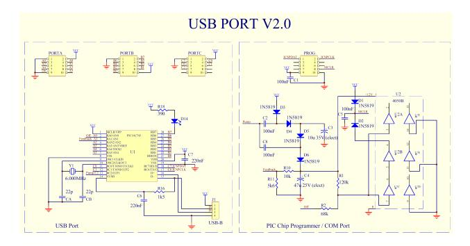
At the heart of the USB PORT Module circuit is the PIC16C745 microcontroller chip. This chip contains all the necessary hardware to implement USB (Version 1.1) Protocol. The chip firmware takes care of all the USB transfers and interprets the commands sent from the PC. The yellow LED (D14) indicates if the USB is active.
