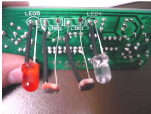
Figure 18: Soldering the LEDs
