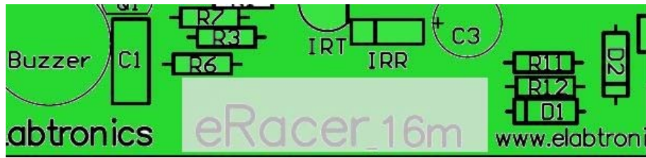
Figure 17: Grey area shows masking tape to hold LEDs and LDRs for soldering
