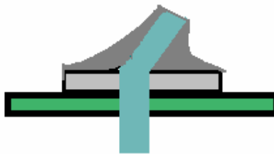
Figure 5: a good solder joint
